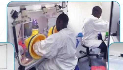
Closed, under-pressured biosafety isolator and BSL-II laminar flow for handling all classes of infectious pathogens that protect both the user and the sample.
