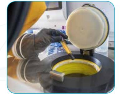
Biohazard waste container safely connected to the inside of the isolator
